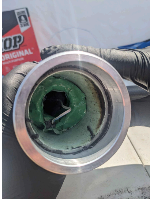
Figure 5.1.3.3.1: Puck igniter used in MACH's first successful hot fire
