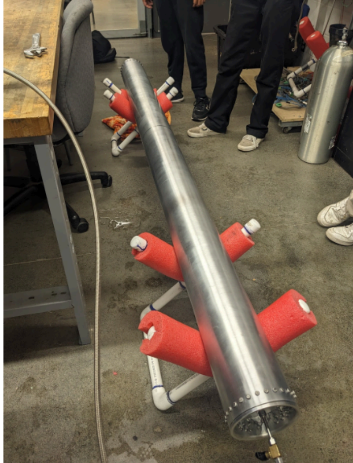
Figure 6.1.2: Nitrous tank hydrostatic test
