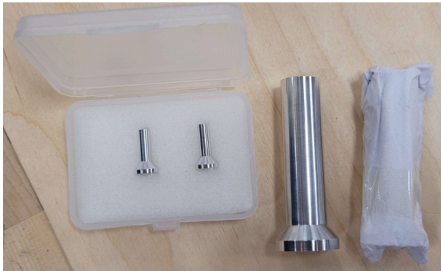
Figure 5.1.2.2.2: SRAD Cavitating Venturis Used for Previous Engine.
