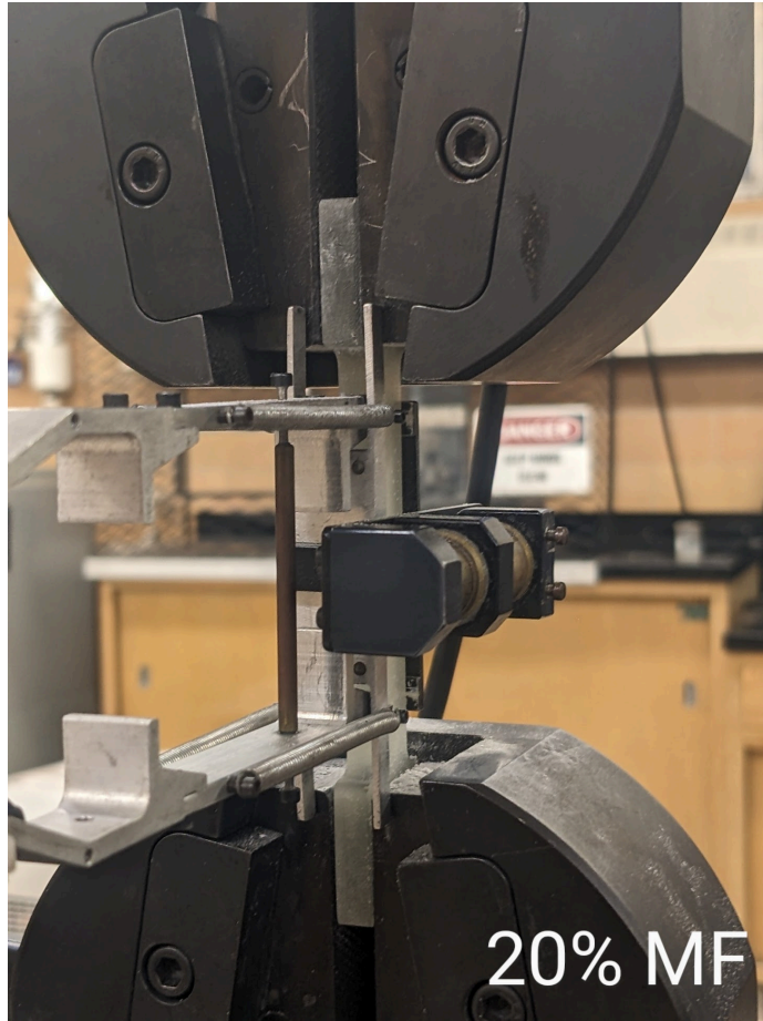
Figure 5.1.3.2.2: Sample undergoing tensile testing ahead of ablative testing.
