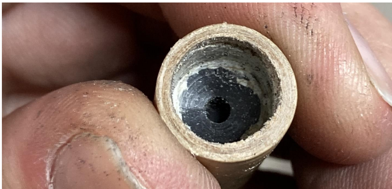
Figure 7.2: Estes A3 with clay nozzle removed (propellant grain exposed)
