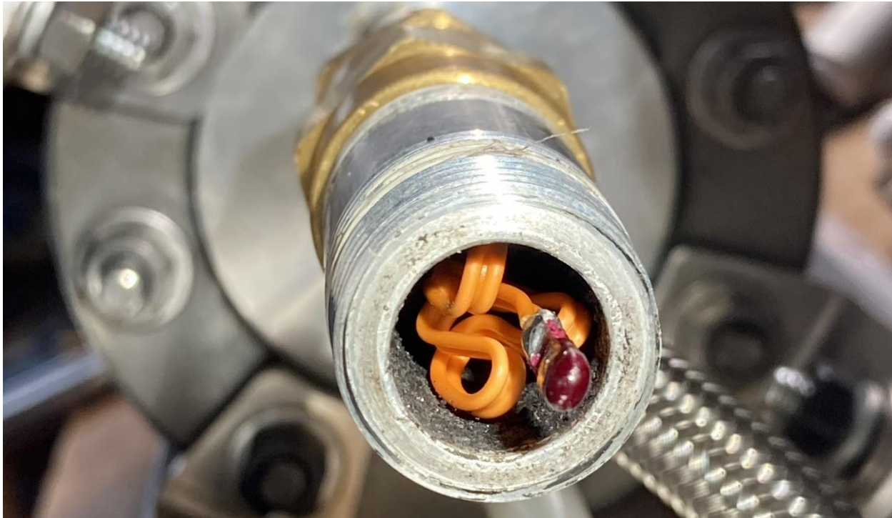
Figure 7.4: Folded e-match inside igniter cartridge
