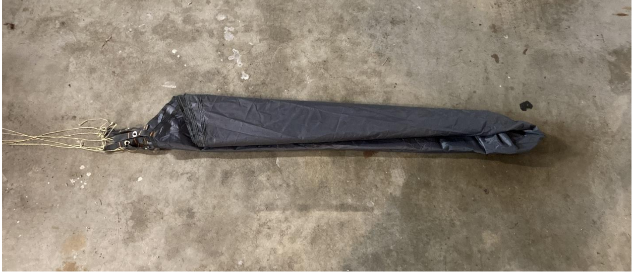
Figure 7.6: Main parachute canopy, folded into strip
