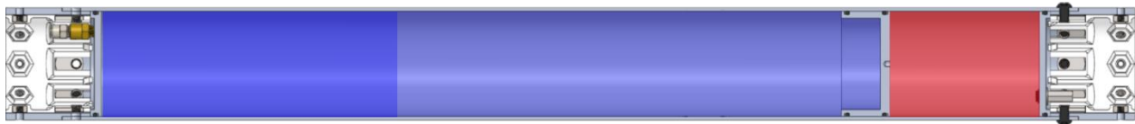
Figure 1.4: Stacked propellant tank with upwards-moving piston (to the right, as pictured), at an arbitrary time during operation. In a stacked tank configuration, the piston moves upwards to force fuel out while oxidizer drains. The drained portion of the tank is replaced by gaseous oxidizer.
