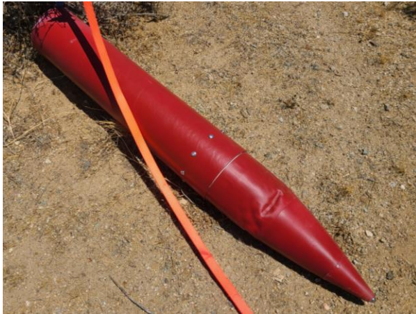
Figure 3.5: Warped PLA+ nose cone
