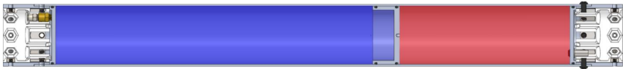
Figure 1.3: Stacked propellant tank with upwards-moving piston (to the right, as pictured), prior to starting operation. Note that in reality, the propellant tank must be upright relative to gravity, so that the oxidizer (blue) drains to the outlet at the bottom (on the left, as pictured) and fuel (red) drains to the outlet at the top (on the right, as pictured).
