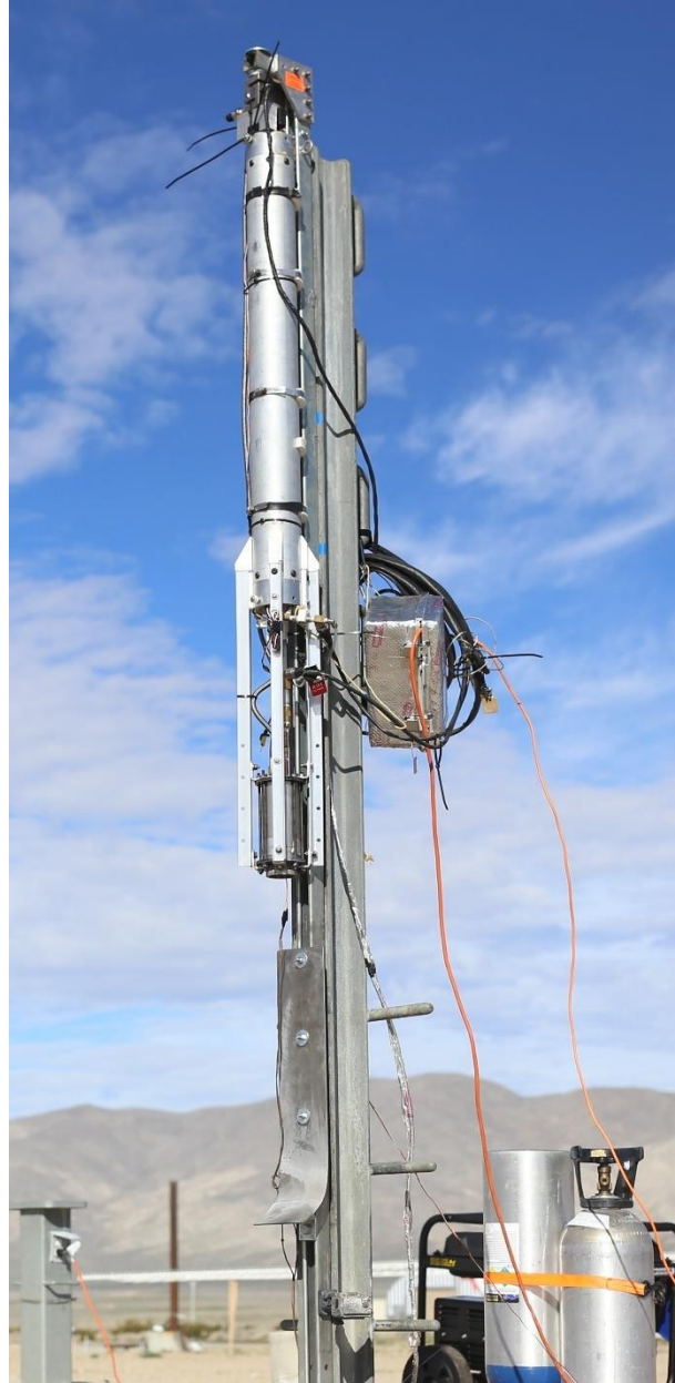
Figure 3.1: Mojave Sphinx in Cat Tower test stand, attached to the FAR medium I-beam
