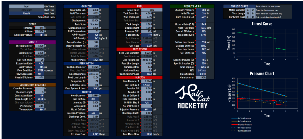
Figure 2.3: Mojave Sphinx HalfCatSim design, motor simulation with basic injector at typical summer temperature
