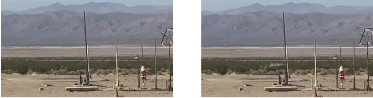
Figure 7.12: Comparison of Mojave Sphinx gas (left) and liquid (right) venting. In this camera view taken from approximately 270 feet away, note how the static vent plume changes from barely visible to a substantial cloud of vapor.
