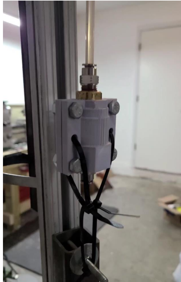
Figure 1.13: Unsuccessful QD mechanism. The printed sleeve holds onto the release ring so that the QD can be pulled out, however in practice the shock load of launch prevented the QD from disconnecting and broke the tether.
