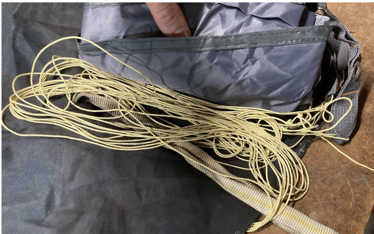
Figure 7.9: Main parachute, laid on protector with shroud lines
