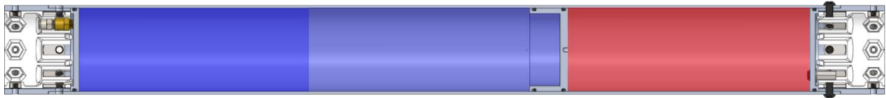
Figure 1.2: Stacked propellant tank with upwards-moving piston (to the right, as pictured), at an arbitrary time during oxidizer fill. The static vent is located just below the oxidizer side of the propellant piston (on the left of the piston, as pictured). Even though the oxidizer tank is sealed, the rocket is hazardous at any time when pressure or oxidizer are present. No personnel are allowed to be near the propellant tank at this point, and must remain away until it has completely depressurized.
