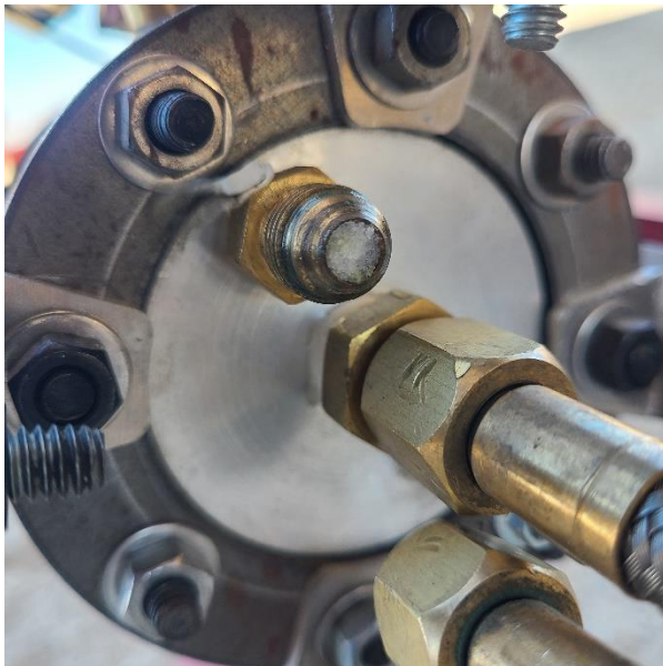
Figure 3.4: Fuel inlet to TCA, clogged with boric acid
