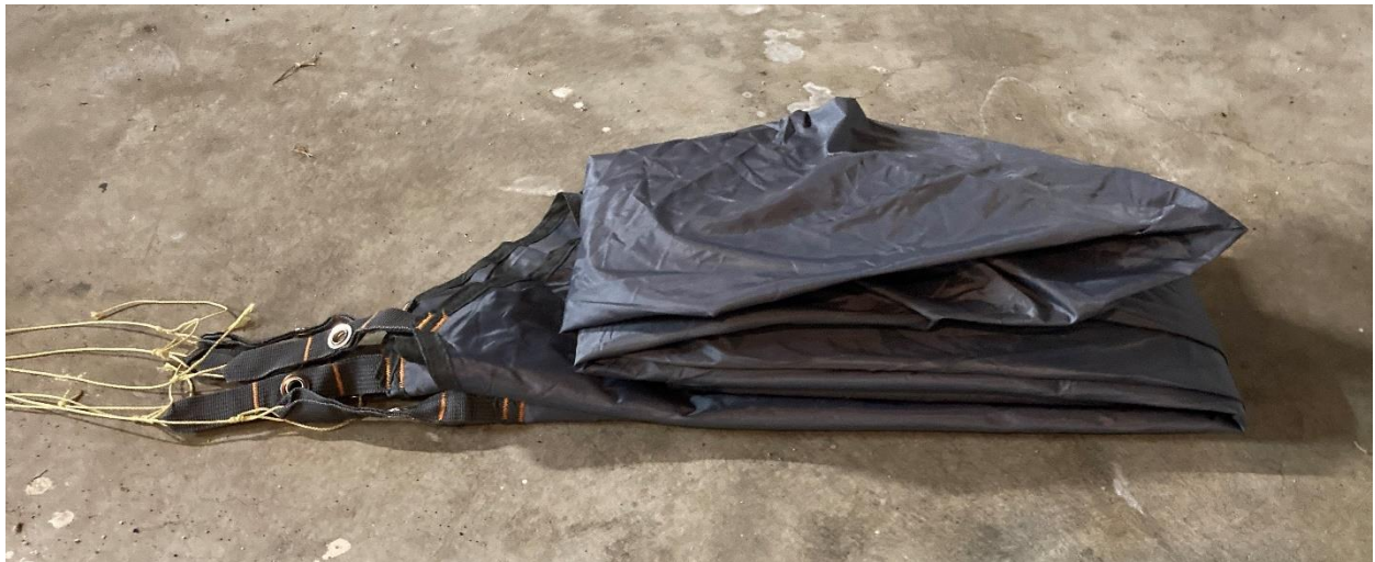
Figure 7.7: Main parachute canopy, Z-folded
