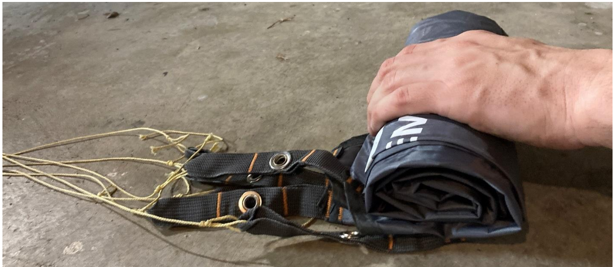
Figure 7.8: Main parachute canopy, rolled into bundle
