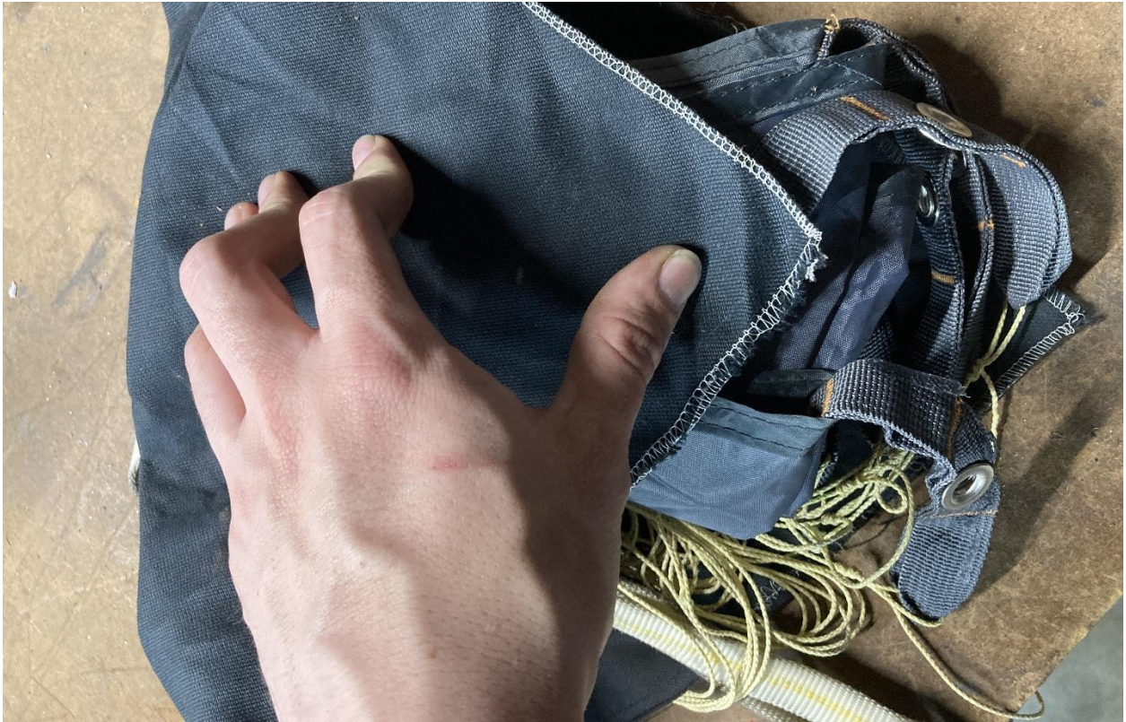
Figure 7.10: Protector folded over main parachute
